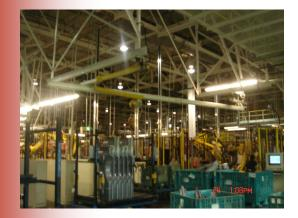
A motor vehicle manufacturer needed to cover a small area inside an existing cell with overhead rail. Ceiling obstructions on one end limited the amount of travel a traditional bridge & runway system would provide, but a broader reach than a single monorail provides was also required.
